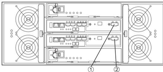
1. Drive Expansion Connector on Controller A
