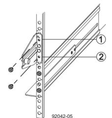
1. Top Cabinet Mounting Hole on the Rear EIA Support Rail
