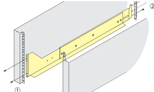
1. Two M5 Screws for the Front EIA Support Rail
