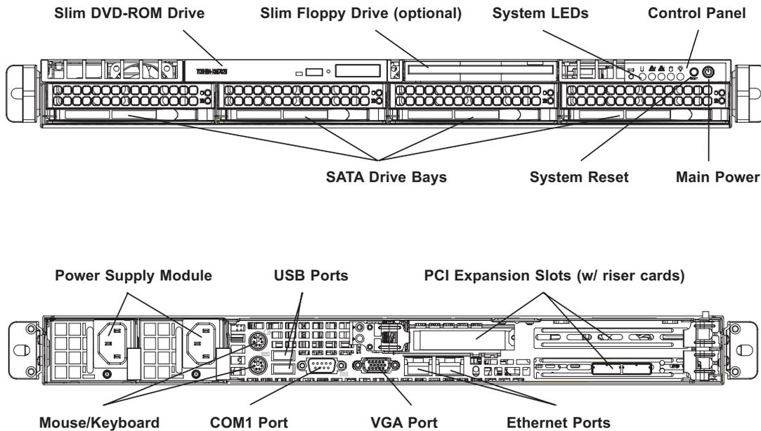
**Note:** the SC815TQ-560U chassis (6015B-U/6015B-NT) has only a single power supply module.
